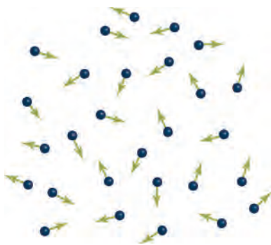
Figure 3.10. Internal energy: The sum of the kinetic energies of the moving particles.
