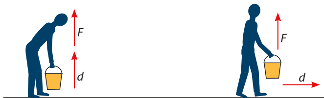
Figure 3.7. In raising the bucket (left), work is done on the bucket. In moving the bucket horizontally, no work is done on the bucket.
